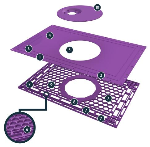
Honeycomb structure provides high specific strength
